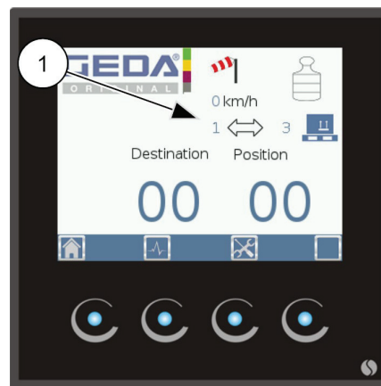
Fig. 53: Display of material transport at ground station
