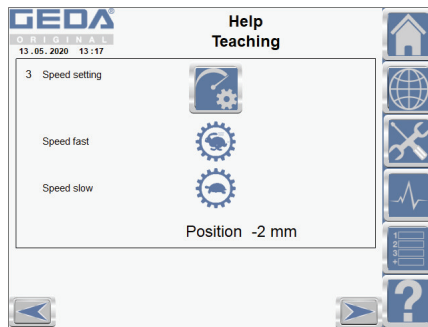
Fig. 14: Programming stop positions 3
