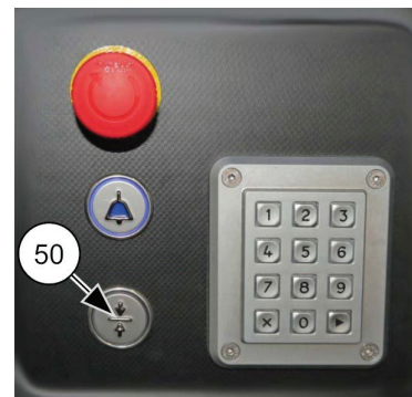
Fig. 23: Key switch in programming mode
