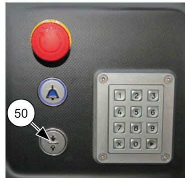
Fig. 25: Deleting stop positions
