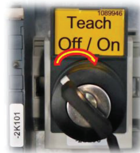
Fig. 23: Key switch in programming mode
