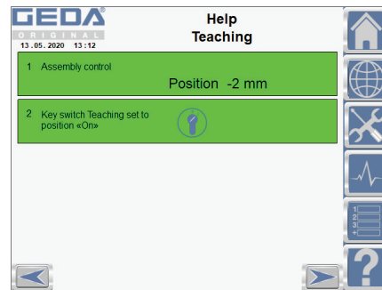
Fig. 13: Programming stop positions 2
