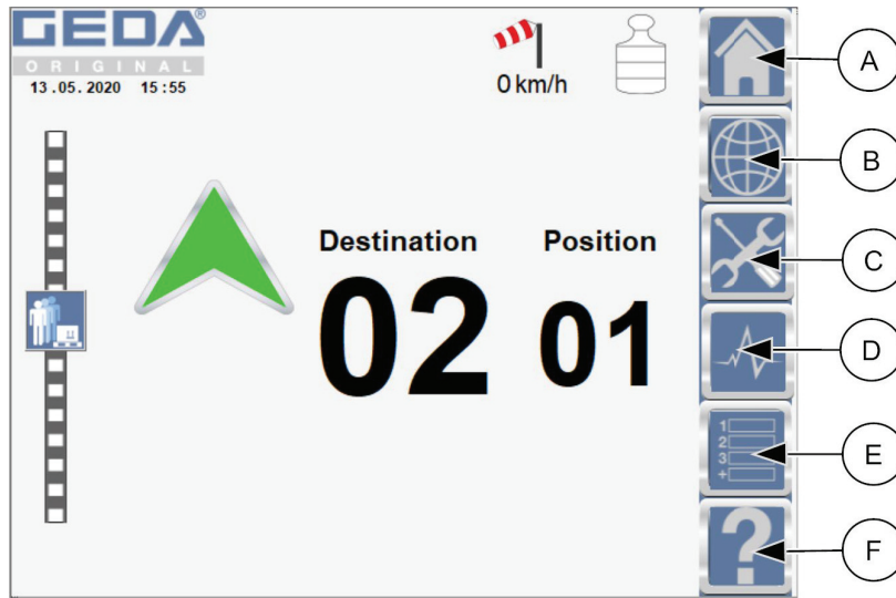
Fig. 2: Touch display (HMI) car 2
