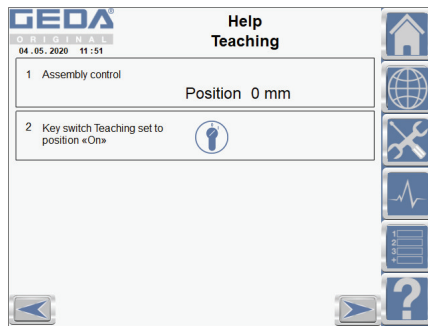
Fig. 12: Programming stop positions 1
